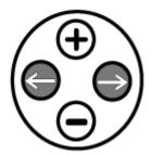
Press either left ( $\leftarrow$ ) or right ( $\rightarrow$ ) control button to access each specific Function page. You can press and hold either button to scroll quickly.
