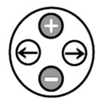
Press either the increment (+) or decrement (-) control button to see/change numeric value of any function. You can press and hold either button to edit numbers quickly.
