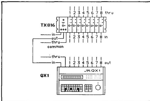
Basic MIDI connections to take advantage of the QX1's new "TX Voice In" and "TX Voice Out" Job Commands when working with the TX816.
