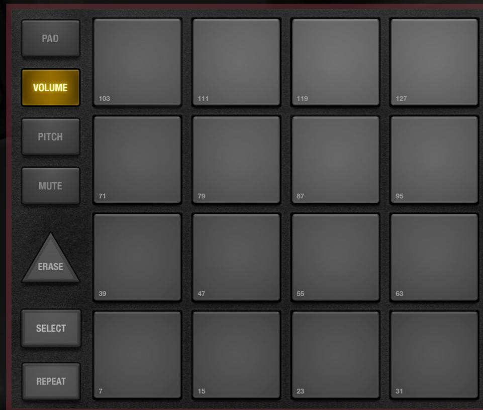
VOLUME mode allows you to trigger a single note at different velocity levels. This is useful when you don't have a proper MIDI controller handy and want to create a dynamic performance.
