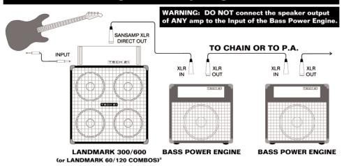
\*NOTE: If you are using an amp that does not have an XLR direct out, use the amp's Effect Loop Send or Pre-amp Out into the Input of the Bass Power Engine. You can then chain or go direct to the PA via the XLR Out of the Bass Power Engine.
