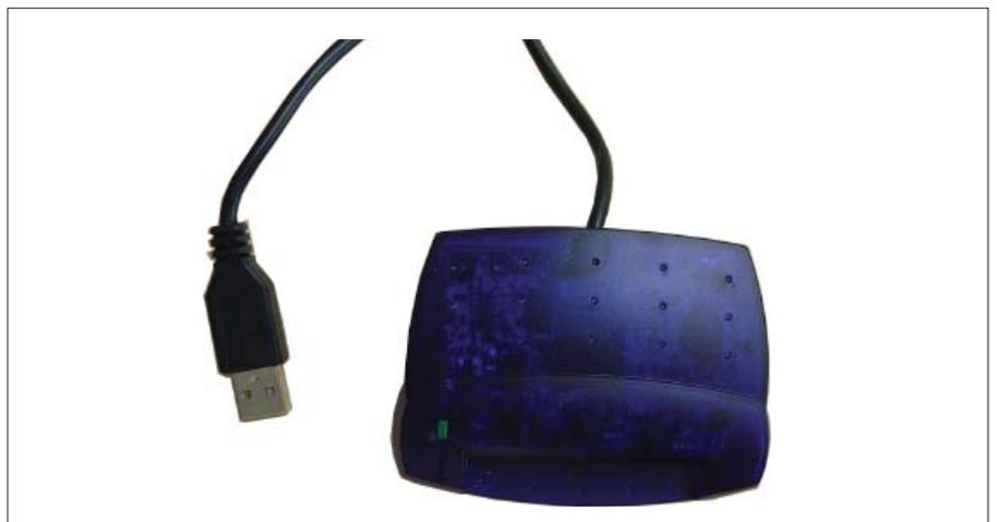
The CP 6000 Chip Card Programmer/Reader is used for programming and reading CC 6010 Chip Cards.
