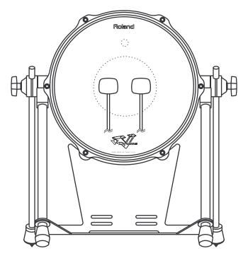
\* When using a twin (double kick) pedal, as with a regular pedal, use the included beater or a plastic beater as the beater for the kick pedal.
