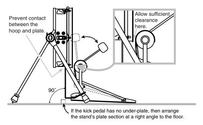
11. Make any fine adjustments necessary and tighten the stand brackets to make sure the KD-120 is secure on the stand.
