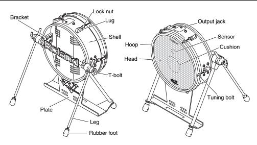
\* Due to the nature of the materials used in the sensor, changes in room temperature and humid may affect the sensitivity of the sensor.
