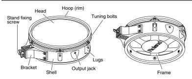
The only difference between the PD-125 and the PD-105 is the diameter.
