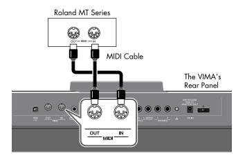
If you connect the VIMA with a MIDI sequencer, turn off the Thru function of the connected MIDI sequencer.
