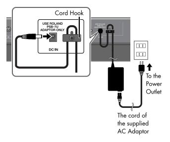
\* To prevent the inadvertent disruption of power to your unit (should the plug be pulled out accidentally), and to avoid applying undue stress to the DC IN jack, anchor the power cord using the cord hook, as shown in the illustration.
