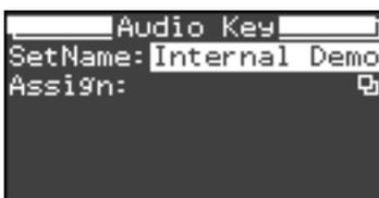
3. While holding down the [Display] button, use the [-] [+] buttons to select "Set Name."
