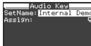
3. While holding down the [Display] button, use the [-] [+] buttons to select "Assign."
