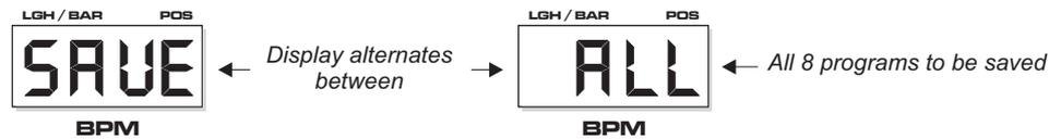
Ensure your connected MIDI storage device is ready to accept the data and then use the NUDGE control 'BPM +/UP' button to transmit all eight programs, as in the following example:
