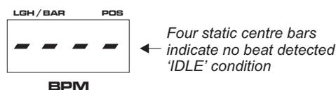
The FEDERATION BPM FX-PRO has two main operating modes for synchronising the effects to the audio. In the first mode the BPM analysis 'engine' is used to calculate the tempo of the incoming audio. This mode can be used for live DJ or studio applications alike. The second mode uses incoming MIDI clock data to constantly define the BPM value which will appeal more to the studio user.
