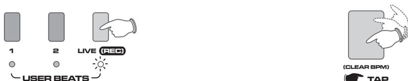
Activate the FILTER (or FLANGER) effect, check the MASTER is set to ON and that the FX MIXER joystick is pointing towards the effect or in the central upright position. Now, use the TAP button to trigger the FILTER effect in time with a particular part within the music, perhaps the bass line.
