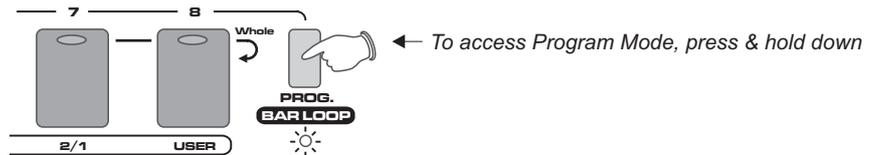
The functions within program mode can only be accessed whilst the 'PROG' button is held down. The labelling above each button designates the program number from 1 to 8.
