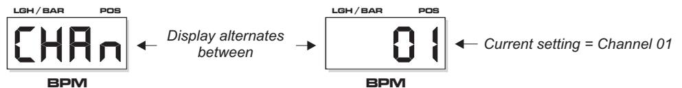
SETTING RANGE = 01 to 16. To change the MIDI channel, use the NUDGE control 'BPM +/UP' or 'BPM -/DOWN' buttons, as in the following example:
