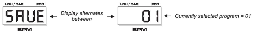
The program displayed, ready for transmission, will be the last selected program (or edited version of the program if changes were made). Ensure your connected MIDI storage device is ready to accept the data then, use the NUDGE control 'BPM +/UP' button to transmit the single program, as in the following example:
