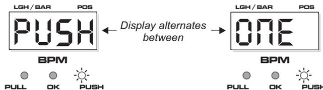
**½ BEAT ADJUSTMENTS:** You can adjust the PULL setting in ½ beat steps by pressing and *holding down* the PULL button for 1 second.
