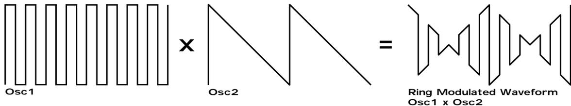
The Ring Modulation effect creates metallic & bell like sounds & is used generally for lead sounds, but if used subtly can produce Electric Pianos etc & if used radically can produce unusual sound effects.
