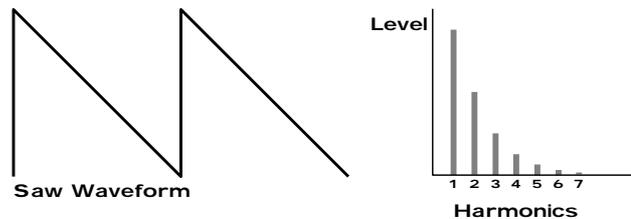
Sawtooth waves have all the harmonics of the fundamental frequency. As you can see, every harmonic has half the amplitude of the previous one. This sound is pleasing to the ear & is useful for basses, leads, & synthesising stringed instruments.
