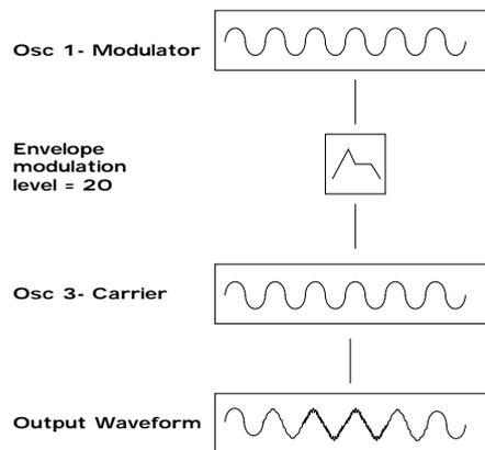
We can see that the output waveform starts off as the same as the carrier, becomes more complex (HARMONICS ARE ADDED) as the amount of FM modulation increases via the envelope, & then returns to a simple wave again as the envelope decays. THE TIMBRE OF THE WAVEFORM IS CHANGING WITH TIME. This is the opposite of subtractive synthesis where often a LOW PASS FILTER is used to REMOVE HARMONICS.
