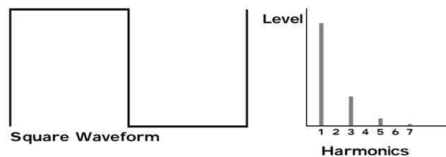
Square waves have only the odd harmonics present. These are at the same amplitudes as the odd harmonics in a saw wave. Square waves have a hollow / metallic sound to them & so are useful in creating unusual synthesiser sounds & oboe like sounds.
