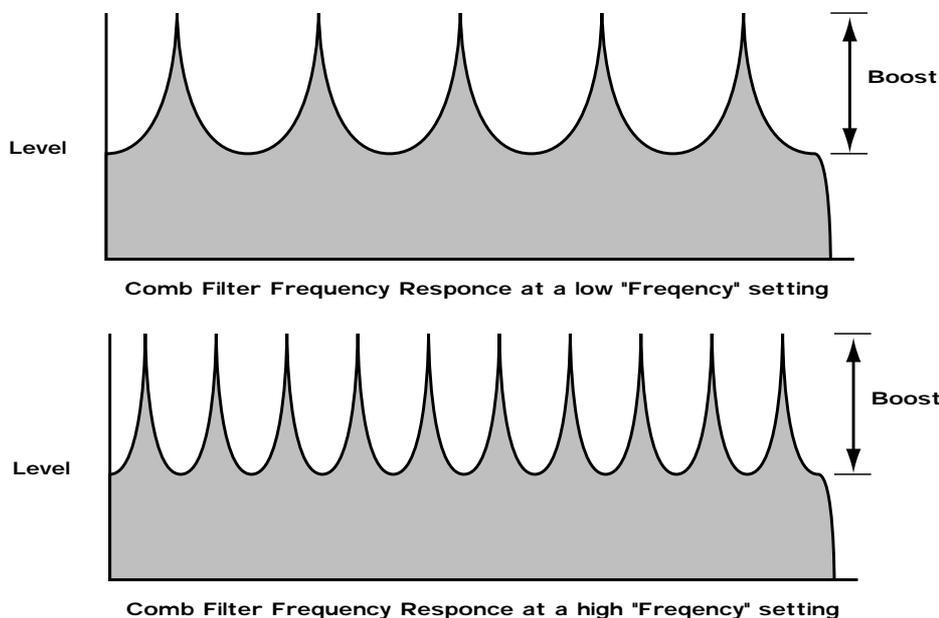
There are many peaks & they look like a "comb" hence the name Comb Filter. There are two parameters associated with this effect. Comb frequency controls the "frequencies" at which the peaks occur & Comb boost controls how high the peaks are. The effect is to alter the timbre of the sound. Although similar to EQ, this effect can produce effects not possible using a standard EQ. The resulting sound tends to be quite "Metallic" sounding especially when large "Boosts" are applied.
