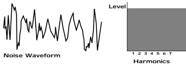
White noise has no fundamental & all harmonics are the same value. This wave can be used by itself to synthesise explosions or wind & when used in conjunction with other waveforms can be used to create the illusion of "Breath" in an instrument.
