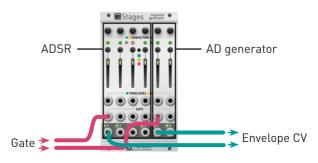
What happens if only **GATE** input 5 is patched? Segments 5 and 6 act as a 2-segment envelope generator; and segments 1, 2, 3 and 4 are four independent free-running generators. Even if these four independent generators do not receive gates or triggers, looping can be enabled for them, turning them, for example, into four LFOs.
