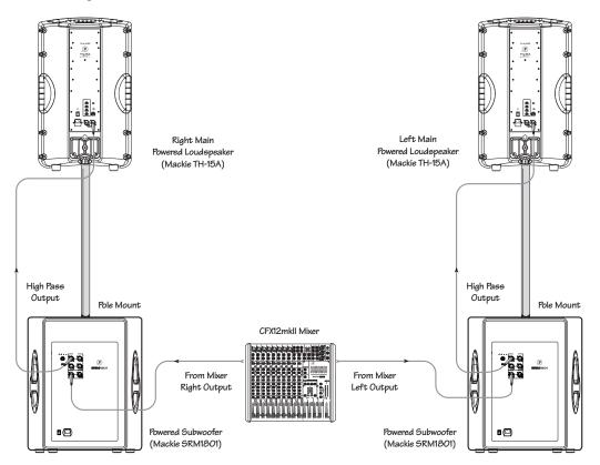
The left and right line-level outputs from a mixer feed the inputs of two powered subwoofers. The high pass line-level outputs of the subwoofers feed the inputs of the Mackie TH-15A loudspeakers.
