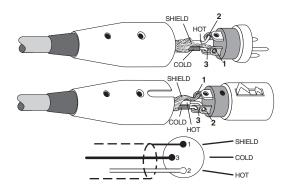
XLR Balanced Wiring Pin 1 = Shield Pin 2 = Hot (+) Pin 3 = Cold (-)
