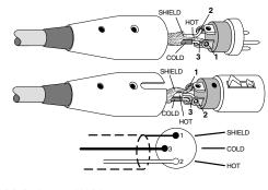
XLR Balanced Wiring Pin 1 = Shield Pin 2 = Hot (+) Pin 3 = Cold (-)
