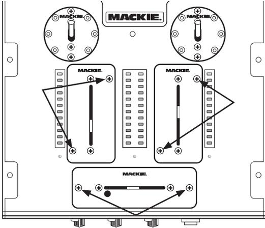
14. Secure the fader assembly to the chassis with the two screws you lost in step 11.
