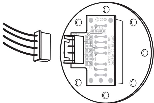
9. Replace the top cover, and make sure that all the meter LEDs and the Reverse LEDs are poking through before you tighten down the screws securely.
