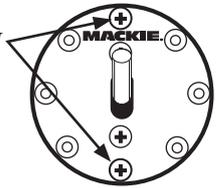
7. Rotate the switch assembly to suit your preference, and replace the two screws.
