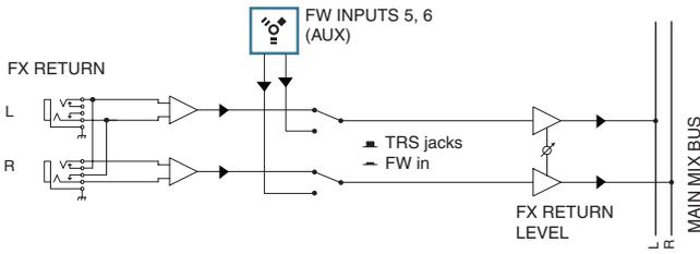
Figure 2: FireWire from computer to main mix
