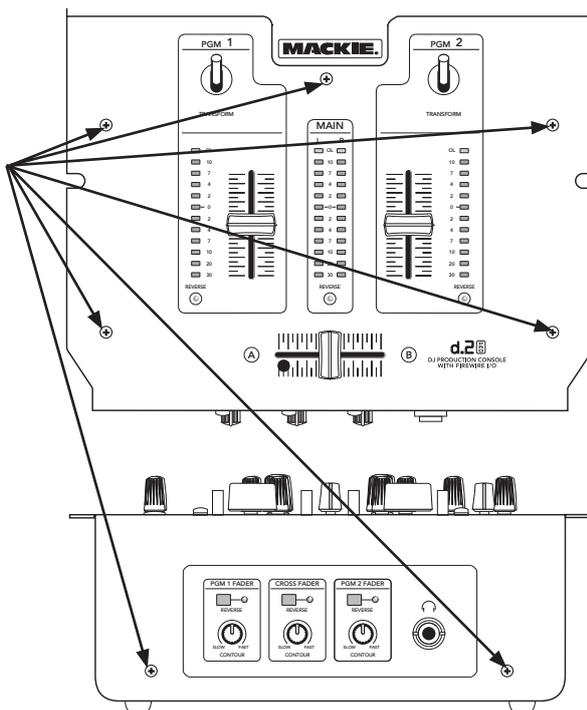
5. Gently lift off the panel, taking care not to damage the front panel contour knobs. Keep it in a safe place where it won't get scratched, or fall off the table.
