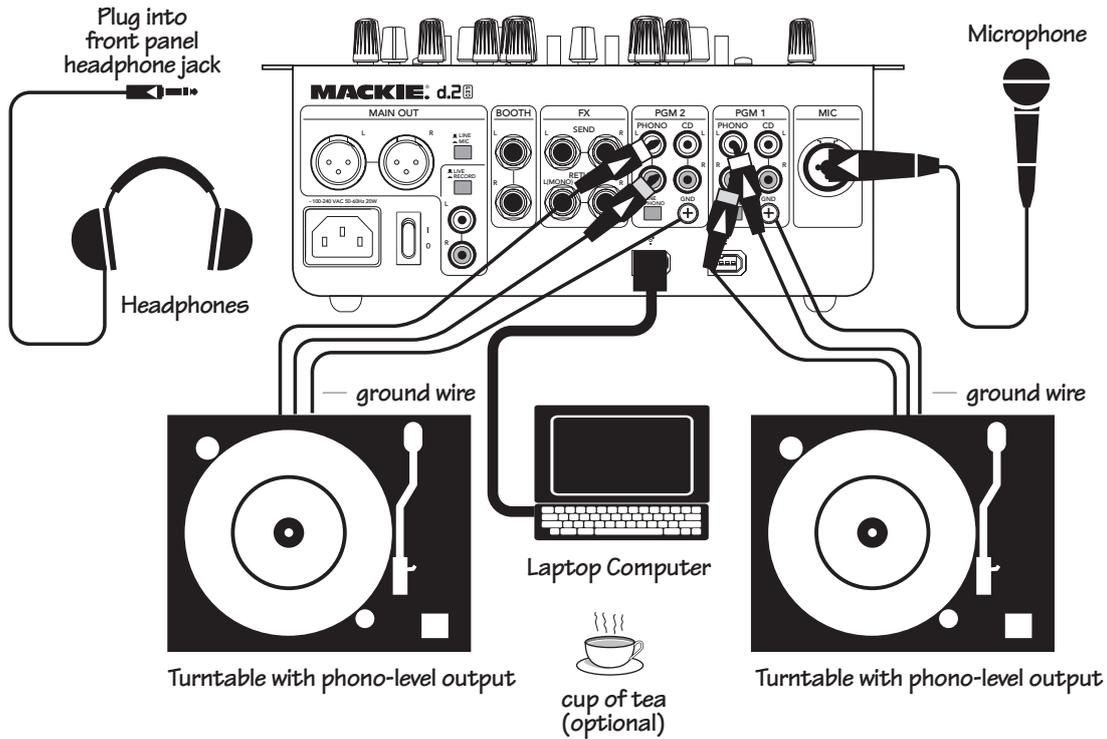
This diagram shows two turntables and a microphone, with the laptop connected for recording and playing.
