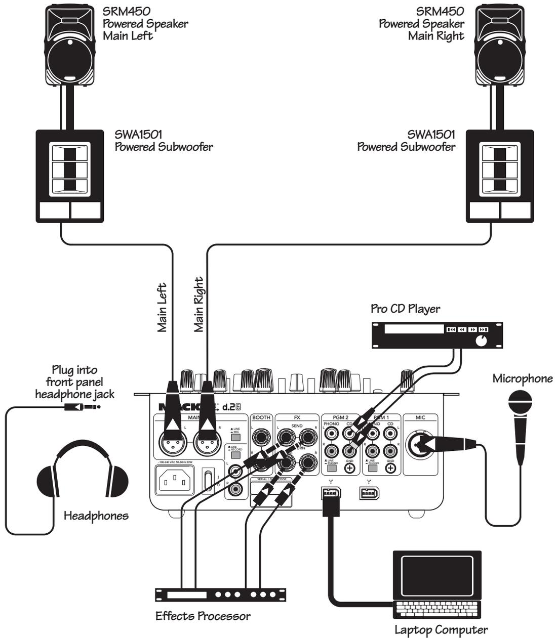
This diagram shows a CD player and microphone connected, with an effects device in the FX loop, and a laptop attached. Various popular DJ software such as Traktor™, PCDJ™, and MixVibes™, can be used with the d.2 Pro via the Fire Wire connection. The main wonder mix can be recorded with software such as Tracktion.
