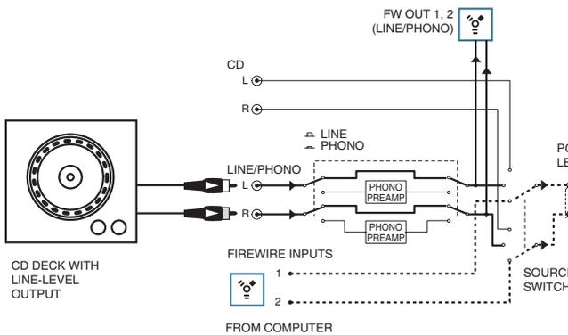
Figure 2: Direct FireWire output from CD deck
