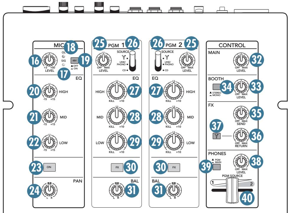
Leave it pressed out if the wet return signals come into the FX return jacks [7] from an external processor.
