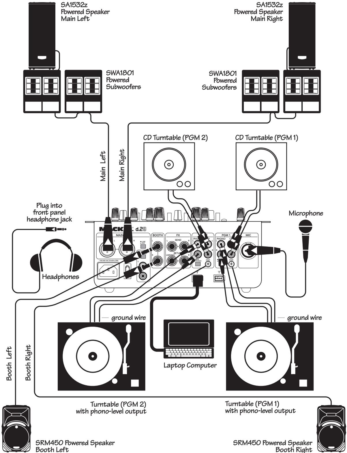
Here the d.2 Pro inputs are fed with conventional sources, and the FireWire connection is used to record the master mix output to computer, using the included Traktion software (for example). The program channels can also be recorded to the computer separately, for added flexibility later in working with the recorded performance. The source select switch can be used to quickly select either the turntable, CD deck, or FireWire as the input to program 1 or 2, without the need for repatching.
