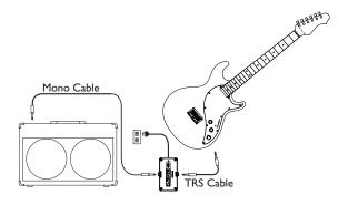
**NOTE:** If you have batteries installed in your Variax, they will be bypassed when using your XPS. If the guitar is connected to the XPS and the XPS power is disconnected, any batteries installed in the Variax will be drained.
