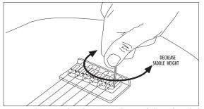
Variax leaves the factory adjusted for playability across a wide range of playing styles. The bridge saddle height can be adjusted to optimize playability for a particular style. If you are familiar with this kind of adjustment, use the supplied Allen wrench to raise or lower the bridge saddle screws as shown. As with neck adjustment, if you are unfamiliar with this kind of adjustment, ask your local guitar shop to refer you to a qualified guitar tech.
