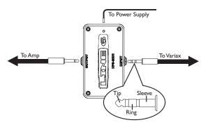
Powering your Variax with the XPS is easy. Use the included TRS cable (meaning "tip-ring-sleeve" or also simply known as a "stereo" cable) to connect the Variax to the INPUT jack of the XPS. Connect the power supply to the XPS POWER jack, and use a standard mono guitar cable to connect the XPS's I/4" OUTPUT to your amp or effects.
