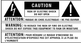
The symbols shown above are internationally accepted symbols that warn of potential hazards with electrical products. The lightning flash with arrowpoint in an equilateral triangle means that there are dangerous voltages present within the unit. The exclamation point in an equilateral triangle indicates that it is necessary for the user to refer to the owner's manual.
