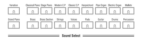
The Sound Select portion of the front panel contains buttons used for selecting the individual sounds available on the RE-220 Digital Piano. You select a sound by pressing the corresponding button; the light in the button illuminates to show you which sound is selected. There are 17 Sound Select buttons. On power-up, the Grand Piano is selected.
