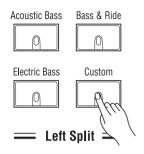
The buttons in the Left Split section of the panel allow you to "split" the keyboard into two parts. Splits are an easy way to make one performer sound like two. When you play the keyboard, your right hand plays one sound and your left hand plays another.
