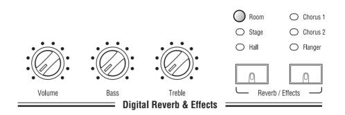
The Digital Reverb & Effects section of the panel contains controls that affect the sound of the instrument as a whole.
