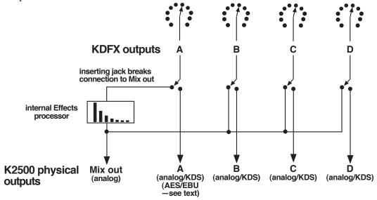
Figure 3-9. Analog, KDFX, and AES/EBU outputs
