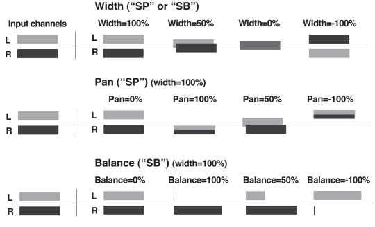
Figure 3-3. Width, Pan, and Balance controls
