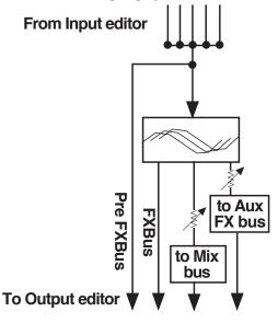
Figure 3-4. FXBus signal routing
