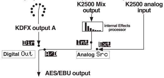
Figure 3-10. AES/EBU output configuration.
