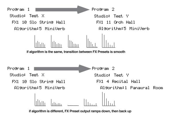
Figure 4-1. Transition between different FX Presets with the same and different Algorithms
