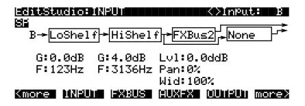
This is the flute, coming from the Program's "KDFX-B" outputs. It is also stereo. The incoming signal has some treble boost on it. It is sent directly to FX Bus 2 at unity gain and full width. Play on the flute part of the keyboard, and the arrow next to "B" flashes.
