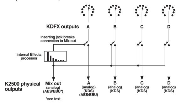
Figure 6-1. KDFX and the K2500's physical outputs
