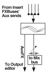
Figure 3-5. Aux bus outputs
