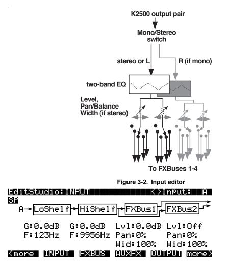
Inputs are referred to as A, B, C, and D, and correspond to the four output buses (KDFX-A through KDFX-D) from the K2500's VAST Program editor. These signals can be treated as stereo pairs or as individual mono signals. This is determined by the first parameter on each Input page, the Mono/Stereo switch.
