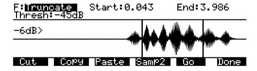
The Truncate function automatically resets the Start (S) and End (E) points of the sample. This can be quicker than trimming the sample manually on the TRIM page.
