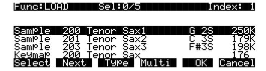
The objects in the list are usually grouped by type (sample, program, keymap, etc.) The list can be scrolled using the Alpha Wheel or the Up/Down cursors. The CHAN/BANK buttons on the front panel can be used for fast scrolling.
