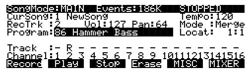
Notice that the R on the Track line, which stands for Record, has moved to Track 2. Also notice how each of the sixteen tracks has a default channel associated with it. You could change this if you wanted to, but most people find it easiest to associate Track 1 with Channel 1, Track 2 with Channel 2, etc.
