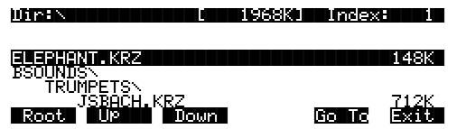
The Dir (Directory) parameter shows the directory that is being listed. The size value displayed on the top line of the display represents the total size of the directory subtree that is currently being viewed. The **Root**, **Up**, and **Down** soft buttons control going from one directory to another in the hierarchy:
