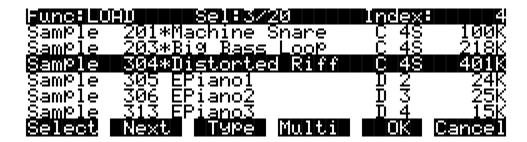
The **Next** button will cause the index into the list to jump to the next selected object, forward in the list. When the end of the list is reached, the search will wrap around from the beginning. If you have more than one object selected, then if you repeatedly press **Next** you can easily cycle through all selected items. If there are no items selected, then this button doesn't do anything.
