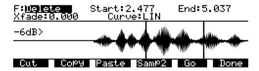
Unlike the Clear function, Delete erases the samples within the selected range and shortens the sample, like cutting a section out of a tape and splicing the ends. If you want to silence a segment of the sample without shortening it, use the Clear function.
