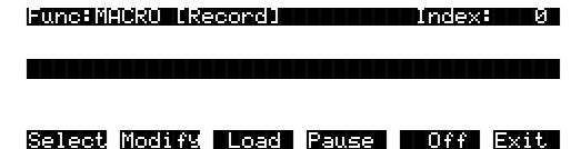
The new macro mode is displayed ([Record]), and the soft button that used to say Record now says Pause. The soft button that used to say On now says Off. Pressing Pause will cause the macro mode to read [Pause] and the Record soft button to reappear. You can switch between Record and Pause by pressing this button repeatedly.
