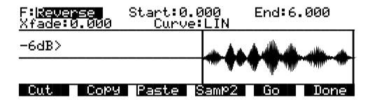
With this function you can reverse the order of the individual samples between the start and end positions you set. The Xfade parameter lets you apply a crossfade to the start and end of the reversed segment. The Curve parameter lets you select a crossfade curve. The available values are LIN, EXP, COS, EQL, and MIX. See *Crossfade and Volume Adjust Curves* on page 2-29 for more information about these curves.
