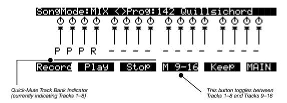
Use the **M 1-8** / **M 9-16** soft button to determine which tracks are affected by the mode buttons: either 1–8 or 9–16. In the preceding display, Tracks 1–8 are affected by the mode buttons, and the **M 1-8** / **M 9-16** soft button displays **M 9–16**. If you press this soft button, the Quick-Mute Track Bank Indicator moves to indicate Tracks 9–16, and the soft button changes to display **M 1–8**.
