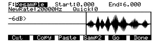
Use this function to change the sample rate of the samples in the selected segment. This is convenient for converting samples to new rates matching those of other samples to be mixed with or inserted into. It's also useful for saving memory and altering the timbre of a sample. To resample so that you'll hear a higher pitch for the same note, select a lower sample rate. For a lower pitch at the same note, choose a higher sample rate.
