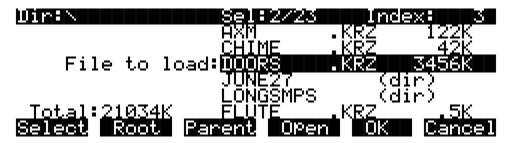
Typing a number on the K2000 alphanumeric buttonpad will automatically scroll the display to the corresponding entry in the file list. Typing an out of range value such as **999** is a quick shortcut to get to the end of the file list.
