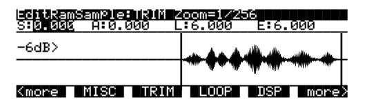
The four parameters on this page are Start (S), Alternative Start (A), Loop (L), and End (E). Selecting these parameters and adjusting their values enables you to modify how the sample plays back when notes are triggered.
