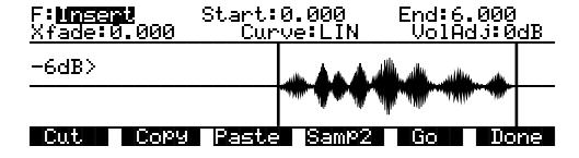
Use this function to insert the selected segment from Sample 2 into Sample 1. This is like splicing a section of tape into an existing tape. This differs from the Mix function, which merges the two samples into one.
