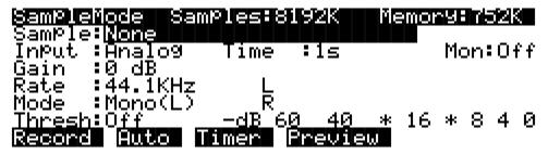
The digital meters at the lower right of the display give a good indication of your sample level. When you send a signal from your sample source, you should see the meters respond.
