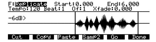
The Replicate function is similar to the Mix Beat function—with two differences. The primary difference is that the Replicate function uses the selected Sample 2 segment to overwrite (replace) the selected Sample 1 segment, instead of merging the two segments like the Mix Beat function. This makes it run faster. The other difference is that there is a crossfade parameter instead of a Volume Adjust parameter. The crossfade parameter lets you smooth the transition points from Sample 1 to Sample 2.
