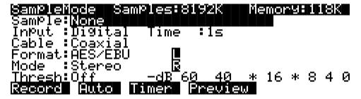
The first difference is the fact that there are no parameters for gain and sample rate. There's no need for a gain parameter because with digital sampling, since you're making an exact digital copy of the source signal. The Rate parameter is excluded because the K2000 automatically recognizes the source sample's rate and sets its own rate accordingly. Also, the Mon parameter
