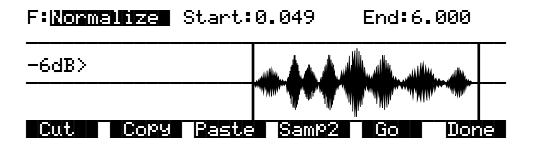
All of the DSP functions operate on a segment of the current sample that you select before executing the function. In most cases, you'll use the Start and End parameters to define the start position and end position of the segment you want to modify. There are a few exceptions to this rule, which will be explained as applicable.
