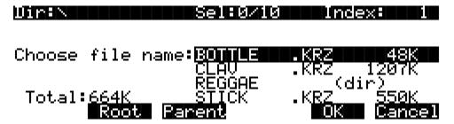
The function of this dialog is to grab the text of any file name on the current disk, and either use it as a starting point in the file naming dialog, or else use the chosen filename exactly. This helps when replacing files on the disk (where the name must exactly match the file being replaced), or adding files to the disk that have similar names or appended revision numbers. You can save time by not having to type the entire file name in from the K2000's keypad.
