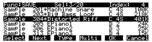
The **Next** button will cause the index into the list to jump to the next selected object, forward in the list. When the end of the list is reached, the search will wrap around from the beginning. If you have more than one object selected, then if you repeatedly press Next you can easily cycle through all selected items. If there are no items selected, then this button doesn't do anything.
