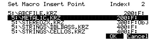
Scroll the macro list until the entry before which you want to insert is highlighted. In the above display, any new macro entries added by this load operation will be inserted in the macro list just before the entry for **METALIC.KRZ**.
