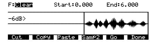
The result of this function is like erasing a section of recording tape. Use it to create sections of silence without changing the overall length of the sample. If you want to completely remove a segment and shorten the sample, you can do it with the Delete function.
