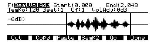
This function works much like Mix Beat. The difference is that you're not mixing in any samples, you're just volume adjusting Sample 1 at regular intervals. Each beat is adjusted in volume by the amount specified for the VolAdj parameter. This is useful for mixing part of a sample within itself.
