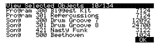
The top line shows 10 objects selected out of 134 that are in RAM. If the number of selected objects is larger than the 6 objects that fit on one screen (as in this example), the list can be scrolled to view all of the information.
