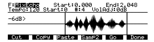
This function operates much like Mix Beat, but instead of the Beat and Of parameters, you have Start and # (number) parameters. The Start parameter sets the beat at which the selected Sample
