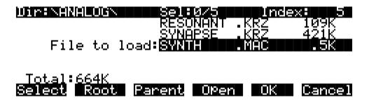
The K2000 will need to read the macro file into a temporary area of internal memory, which means there needs to be enough free RAM to accommodate it. When **Open** is pressed from the Load function, a dialog similar to the MACRO page and the Save Macro page will be entered, called the Load Macro page:
