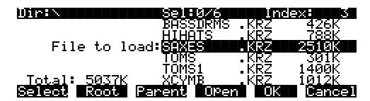
Press **Open** to begin the Load Object dialog. (Note: The file must have a **.KRZ** extension in order to load individual objects from it.) The K2000 then scans the file contents in order to present a list of all of the objects in the file. Sometimes this procedure can take a few moments, depending on how many objects are in the file. During this time, you will see the following display:
