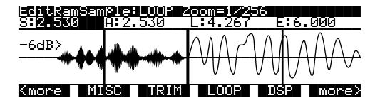
On the TRIM page you see the entire waveform—or as much of the waveform as your current zoom setting allows. When you move to the LOOP page, you'll notice that the page is split into two sections, left and right, divided by a vertical bar in the center. This bar is thicker than the vertical lines representing the Start, Alt, Loop, and End points, and does not move when you adjust any of these points.
