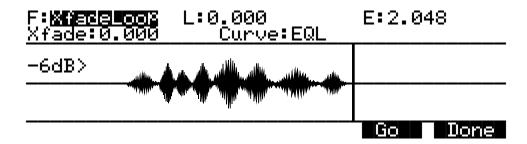
The Crossfade Loop function lets you create smoother loops by crossfading the beginning segment of the loop with a segment of equal length at the end of the loop. These segments can be defined by the Loop and End parameters as set on the TRIM or LOOP page for the current
