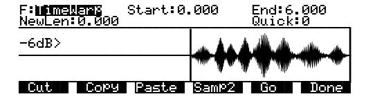
With this function you can change the length of the selected sample segment without affecting the pitch. This function applies sophisticated routines that lengthen or shorten the selected sample segment to play it back over a different time period, modifying the playback rate so the pitch remains unchanged.
