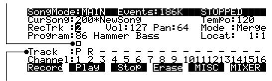
This line contains the track status indicators. In this case, Track 1 is a playback track, Track 2 is the recording track, and Tracks 3–16 are empty.
