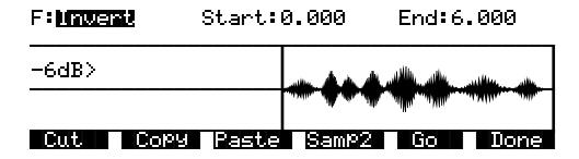
Use this function to invert the waveform of the selected sample range. The results will vary depending on the type of sample. For an interesting phase effect, make a copy of a sample, then invert the copy, then assign it to the keymap of a second layer in a program that uses the original sample in the keymap of the first layer (or set them as the Left and Right samples in a stereo keymap). Add a delay to one of the layers or keymaps to create the phase effect.
