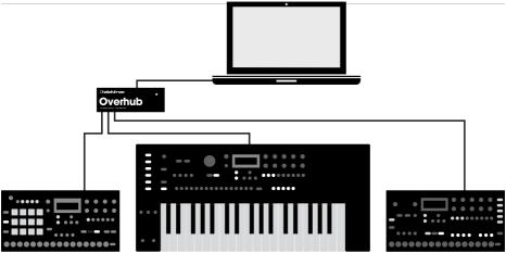
The Analog Keys is a highly capable standalone instrument. Since the introduction of Elektron Overbridge, however, there is a complementary way of interacting with it. All that is required is an Elektron Analog instrument, a USB cable, a computer running Overbridge, and a DAW.
