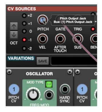
Show Bus Connections- Hovering over any jack with a cable bus temporarily enlarges the colored circles for all other jacks currently assigned to the bus. This makes it easy to see jacks on the selected cable bus.
