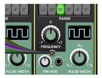
Multiple cables plugged into a single jack can be moved at the same time by holding the [SHIFT] key and clicking and dragging to a new destination. This is also a very handy way to unplug multiple cables from a jack if the mouse button is released in an "empty" area (i.e., not on a jack).
