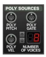
Voltage Modular's Poly modules make use of a special "poly" cable, identifiable by its slight larger D-shaped connector and striped cables. Each poly jack and cable can transmit up to sixteen separate channels, or "lanes," of CV or audio, which drastically simplifies polyphonic patch creation.
