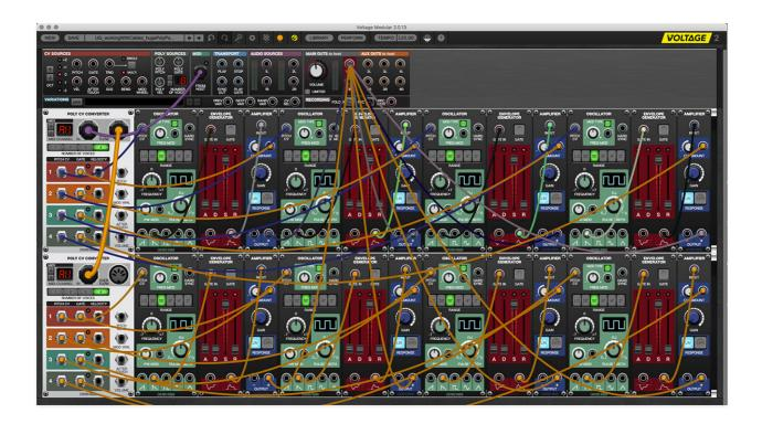
At minimum, a basic polyphonic patch would include an oscillator, envelope and amplifier for each voice. To create eight-voice polyphonic version, that would require 24 modules - something like the hot mess above. Once additional envelopes, filters, modulations etc. are added, it's easy to see how this would make for a huge and hard to control patch. Poly cables and jacks **immensely** simplify the creation of polyphonic patches.
