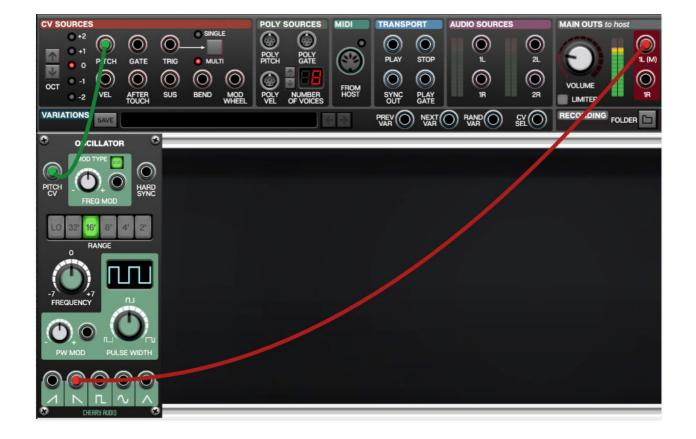
Here we've added two cables for a basic subtractive synth patch. The green cable routes the keyboard pitch control voltage out (we'll refer to control voltages as "CV's" from here on out) to the oscillator's keyboard CV in to allow keyboard control of pitch. The red cable routes the oscillator's sawtooth wave output to the main audio outputs. You'll notice the sound plays continuously, but we're about to fix that.
