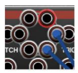
If you look closely at the I/O Panel *Gate* CV out, you can see we've routed two cables from this jack to control both envelope generators. Single-clicking on any Voltage Modular input or output jack reveals a six-way multiple jack (aka, a "mult"), which is super convenient for routing (or mixing) multiple sources. The mult stays visible until a cable is routed, at which point it disappears.
