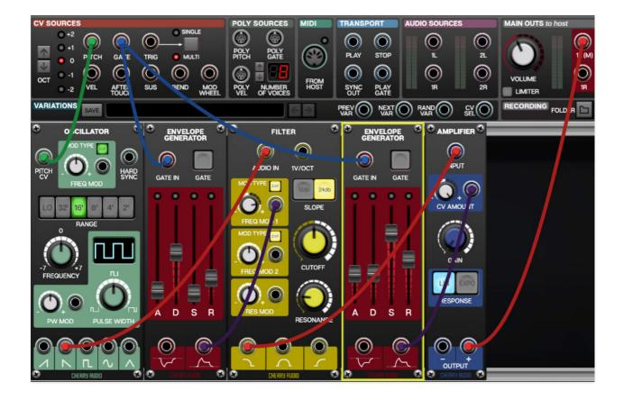
Here we've fleshed out our basic patch with the addition of a Filter, and Amplifier, and two Envelope Generators (one to control the filter cutoff, and another to control amplitude).
