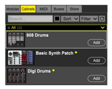
This is a useful Voltage feature that many users aren't aware of. Any cabinet (i.e. a single row of horizontal modules) can be saved *independently of a Voltage preset*. Not only is this is nice for creating patch templates, it's really
