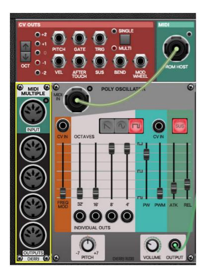
Voltage Modular's virtual MIDI cables behave much like standard cables, but instead of carrying a single audio or control voltage signal, they carry 16 channels of note and control data just like a good ol' MIDI cable. Though virtual MIDI cables have been somewhat superceded by our Poly jacks, they're handy for certain applications, particularly when MIDI controller data is being transmitted or received from hardware instruments.
