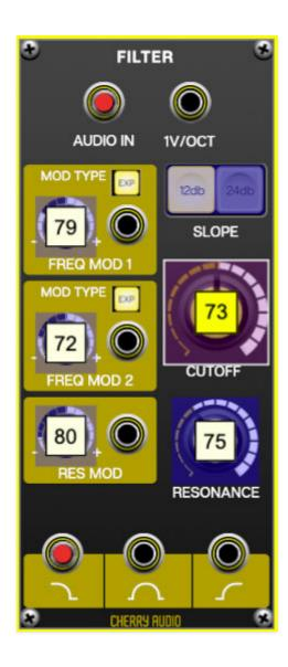
When in MIDI learn mode, previously assigned controls will display numbers in squares on module controls. These indicate the MIDI continuous controller number of the assigned hardware control (these are also displayed in the *MIDI* library tab).
