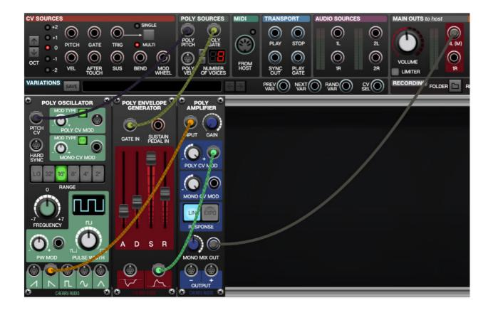
The patch above is more or less functionally identical to our previous "mega patch." It accomplishes the exact same thing with just three modules, as opposed to the other patch's 26 modules. Furthermore, patches made using poly modules and cables can have up to 16-voice polyphony.
