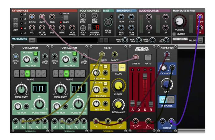
Right-click the I/O Panel *Pitch* jack, move down to *Assign To Mono Bus*, and click *Add New Bus...*
