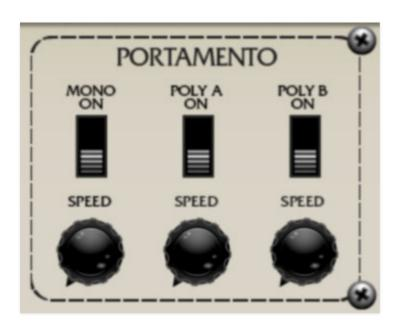
"Portamento" is just a fancy word for glide - that is, instead of notes instantly shifting from one pitch to the next, the pitch change is slurred, like a trombone (only less annoying). Eight Voice includes separate on/off switches and glide speed controls
