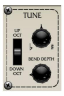
**Transpose switch**- This three-position switch transposes the entire instrument up or down one octave, with the middle position being "normal."
