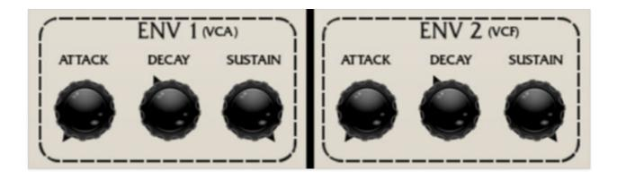
The original SEM modules included two attack/decay/sustain (ADS) envelope generators. These function much the same as more common attack/decay/sustain/release (ADSR) envelopes, the only difference is that the decay and release stages are combined into one control.
