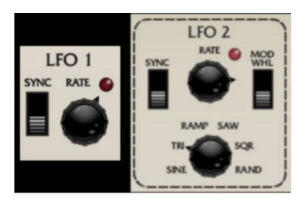
Eight Voice includes two low-frequency oscillator (LFO) that generates subaudio range signals intended for modulation purposes. Actually, Eight Voice has nine LFOs: one for each of the eight voice modules (LFO 1), and a global LFO for the entire instrument (LFO 2). We'll go over LFO 1 and LFO 2 separately as they differ a bit.
