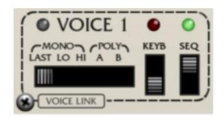
The Seq switch in a voice's voice assignment section (at the bottom left of each voice module) must be enabled for the sequencer to work - if no Seq switches are currently on, the sequencer will run, but it won't be routed to anything. (Don't worry, this won't void your warranty, but the support dept. might give you a gentle ribbing.)
