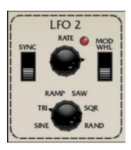
LFO 2 is a global single LFO that can be configured to affect voice mod parameters via the switches in the voice modules. Please see the **LFO 1 and 2** section for more information.
