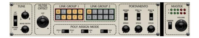
The controls in the bottom section are global, that is they affect *all* voices. These include master tuning, filter offset, voice linking, poly assign modes and more. Note that all master settings are stored individually, per-patch. Some of these sections are covered in other parts of this guide, we'll provide links in those cases.
