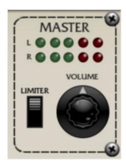
The Master section includes a master volume for the entire instrument and stereo level meters. You'll want to keep this guy out of the red or else digital clipping can occur (which doesn't sound cool). Because Eight Voice is such a beast, sound can easily pile up and get loud - enabling the *Limiter* switch applies a transparent limiting effect to help prevent overloading.
