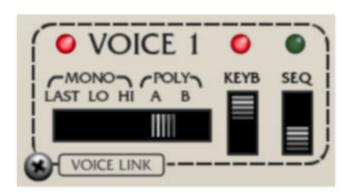
**Voice Active LED**- The LED next to *Voice #* is a bi-color LED that glows red when it's receiving a MIDI note (i.e. note played on a keyboard controller or from a DAW), or green if the note is received from the onboard *Mini Sequencer*. This isn't just another cool flickering light - because of the many
