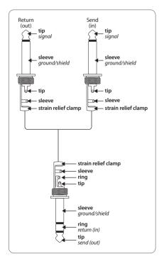
Fig. 4.4: Insert cable with one  $\%^{\rm T}$  TRS (tip-ring-sleeve) jack plug on one end and two  $\%^{\rm T}$  TS (tip-sleevel) jack plugs on the other end.
