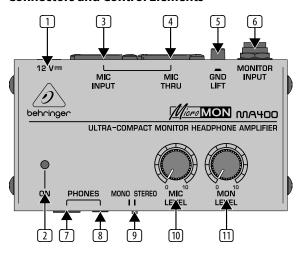
Fig. 1: MA400 connectors and control elements
