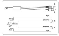
Fig. 4.3: Stereo adapter cable
