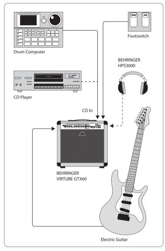
Fig. 3.1: GTX60 standard setup
