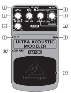
The AM400 has no on/off switch. As soon as you insert the jack into the in connector, the AM400 begins running. When not using the AM400, remove the jack from the in connector. This extends the life of the battery.
