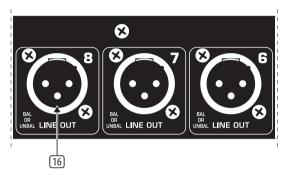
Fig. 2.4: LINE OUT connectors
