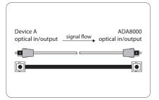
Fig. 4.4: Connecting the ADA8000 optically via Toslink
