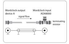
Fig. 4.5: Unbalanced connection (termination) of the ADA8000's wordclock input
