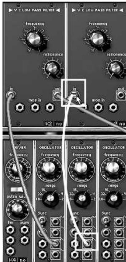
*Connection between oscillator 2 and filter2*
