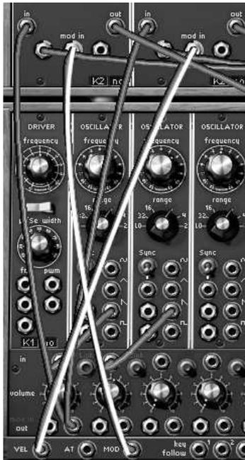
Connections for modulation and velocity outputs on the frequency modulation of filters 1 and 2
