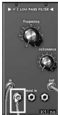
*Turn the modulation jack ring counter clockwise.*
