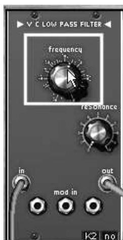
The setting of filter1 cut-off frequency
