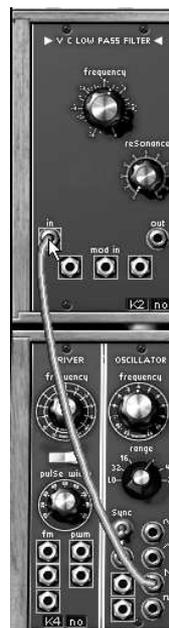
*Connection between oscillator 1 and filter1*
