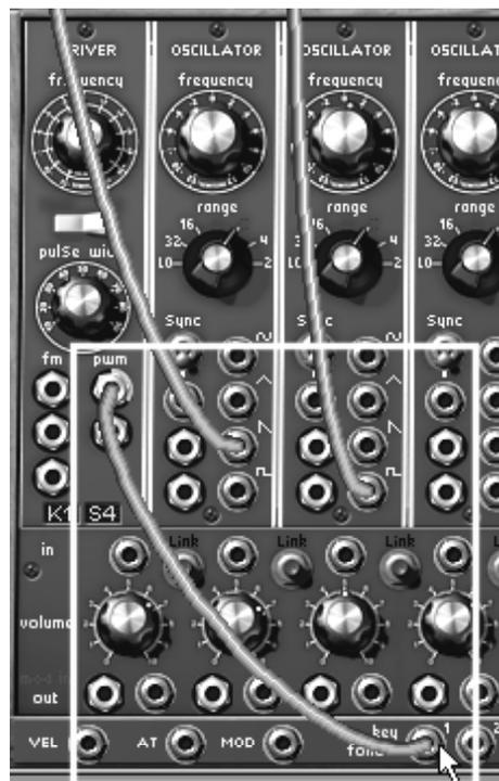
Connection of the “driver” oscillator to the first sequence line
