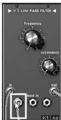
*Turn the modulation jack ring counter clockwise.*
