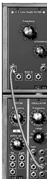
*Connection between oscillator 1 and filter1*
