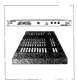
Some mixers are designed to accommodate effects on each input channel via "channel inserts," or "patch points." These often consist of a single 1/4" phone jack acting as both send and return, requiring a dualmono-to-TRS (tip/ring/sleeve) plug configuration. Check your mixer's owner's manual to determine which plug of the dual-mono-to-TRS cable acts as a send, and which acts as a return. If the mixer has individual send and return jacks, simply use two standard cables.
