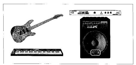
When plugging a guitar, keyboard, or other instrument into the FXR Elite, make sure that there is sufficient signal level coming from the instrument. Pay attention to the Signal LEDs on the FXR Elite's front panel, and use the FXR Elite's input knob and the instrument's volume control to get the best level and signal-to-noise ratio.
